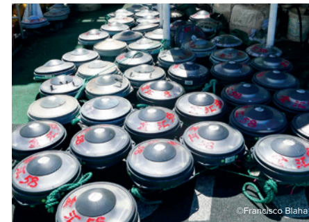
FAD transponders. Each will be attached to a FAD and transmit information about the fish that are present under the FAD, as well as positional location.
