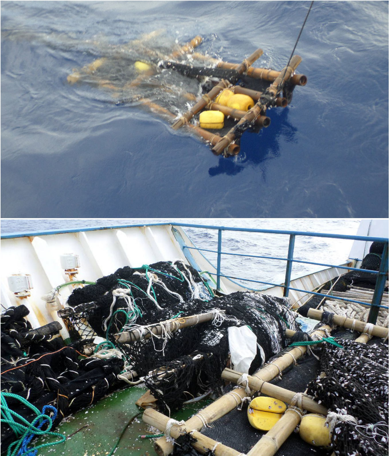
Figure 8: Fish Aggregating Devices (FADs) Being Pulled from the Sea (Top) and on Deck
