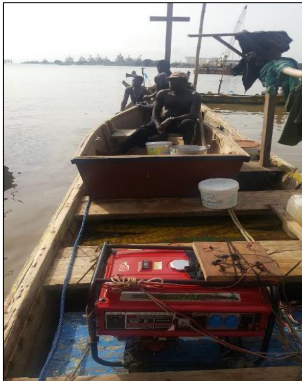
Figure 6. An artisanal canoe carrying petrol-powered generator (in a daughter boat) and 1,000 watt bulb for light fishing.
