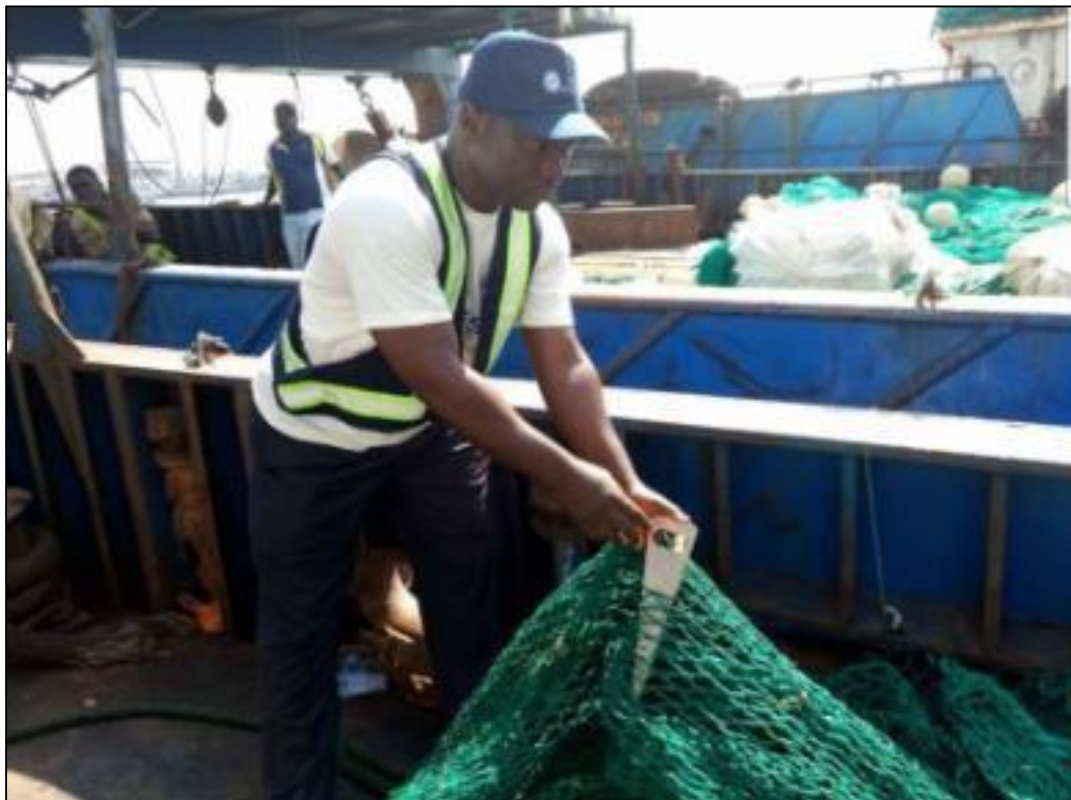
Figure 17. An enforcement officer measuring the mesh size of a fishing net (citifmonline.com)
