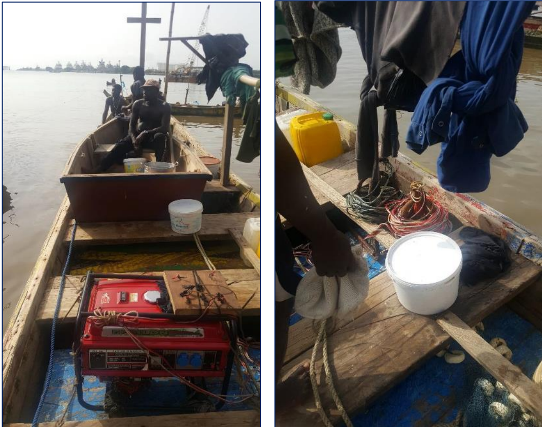
Figure 15. Artisanal canoe carrying portable generator, switchboard and two 1000 watt bulbs
