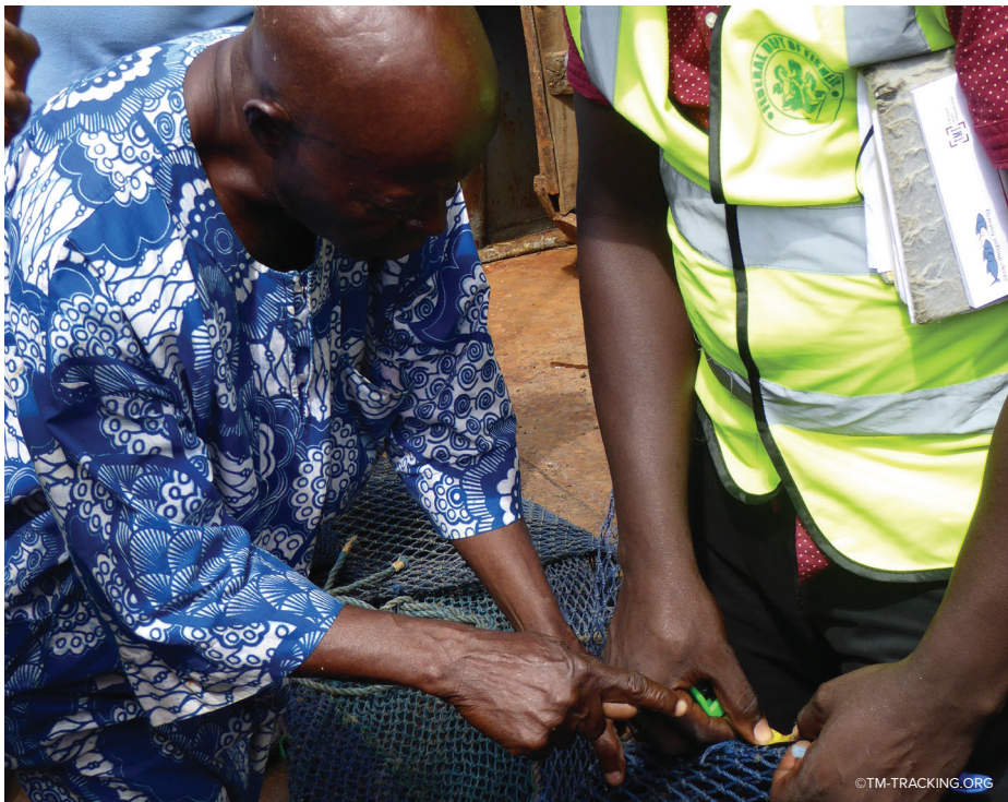
Mesh size, particularly in the cod-end, should always be inspected to ensure it meets regulatory requirements
