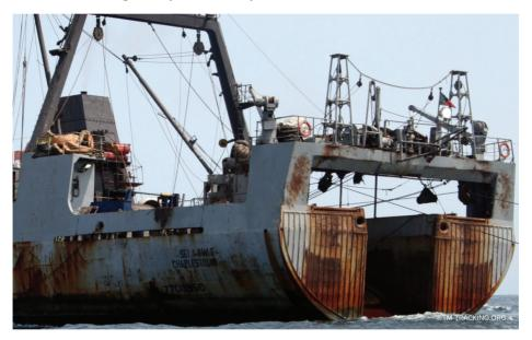
When not in use, otter boards will often be visible at the stern of a trawler (for those that use otter boards). If no doors can be seen, the vessel will probably be trawling, and the warps should be visible running from the towing or trawl blocks into the water astern of the vessel.
