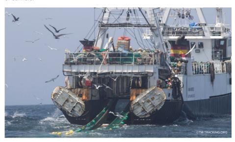
A midwater trawler retracting gear through the stern ramp
