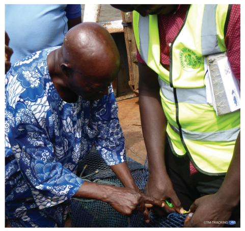
$\textit{Mesh size, particularlly in the cod-end, should always be inspected to ensure it meets \textit{regulatory requirements} \\$
