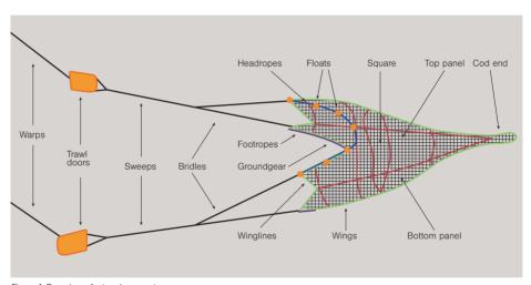
Figure 1. Overview of a trawl gear setup
