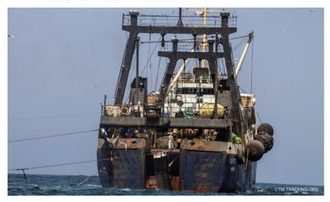
Pelagic or midwater trawling targets fish which school between the surface and the seabed. A midwater trawl works in much the same way a bottom trawl does, but the trawl mouth of a midwater trawl generally has a wider opening. Weights are attached to the bottom sweeps to pull the groundline downwards. Midwater trawls are generally conducted at slightly higher speeds than bottom trawls.
