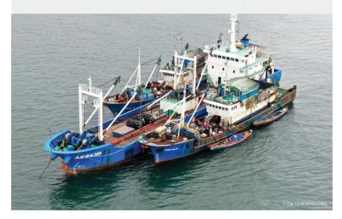
3. In some fisheries, "carriers" may come in the form of other fishing vessels, or even large canoes, but are normally large-sized steel-hulled refrigerated cargo (reefers), ships such as the middle vessel above between two trawlers
