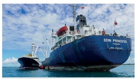
Transhipping at anchor in port area. Note the large 'Yokohama' fender deployed between the carrier and unloading vessel.
