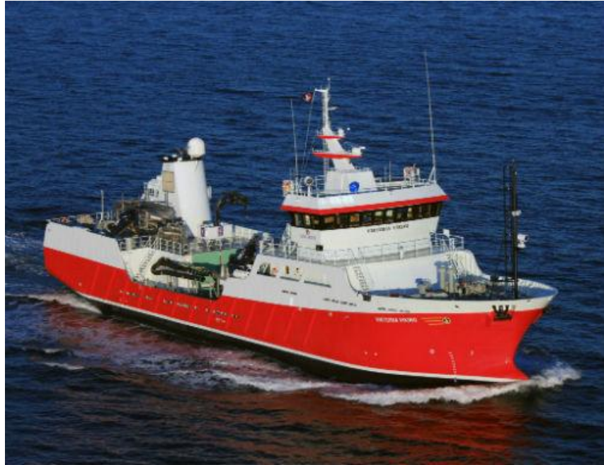
Picture 8: Typical Norwegian-type small scale RSW fish-carrier. ©Dag Remoy-MarineTraffic.com.
