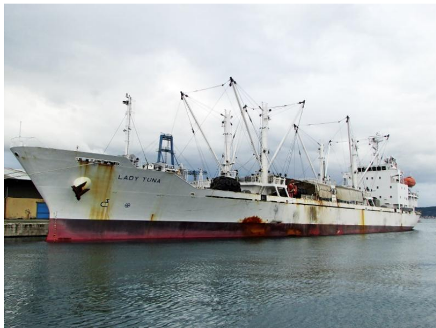
Picture 9: Typical reefer vessel capable of fish-transshipment-at-sea. ©marinko-MarineTraffic.com.
